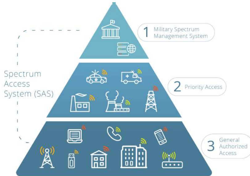
Figure 1: Illustration of real-world proposed Citizens Broadband Radio Service shared spectrum user tiers (from Federated Wireless' spectrum-sharing whitepaper 1 ).
