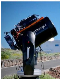
Figure 1. Astrolight portable laser com terminal for satellites
