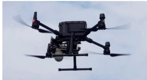
Figure 2. Astrolight 2 \mu m infrared laser com prototype terminal during pilto flight testing
